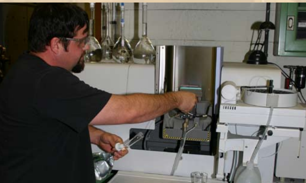
Plant Morrow Lab Technician Bryan Lindley uses an Atomic Absorbance Spectrometer to analyze a sample of process water to determine its concentration of trace metals.
